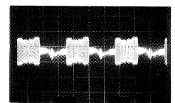
5. IC601 Pin 38 (E-PCB) R - Y In 180mV, 20 \mu s / Div
