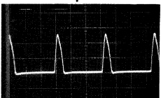
17. Q501 Collector (E-PCB) Horizontal Out 1240V, 20 \mu s / Div
