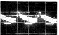
22. IC601 Pin 7 (E-PCB) Vertical 2.1V, 10 \mu s / Div
